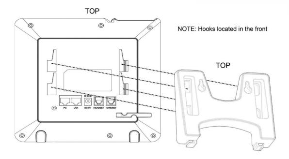
Figure 3: GXP16xx Wall Mount installation
